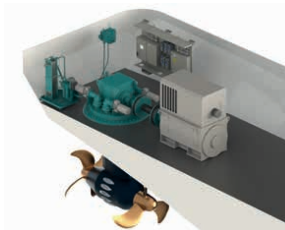
Z-drive with horizontal motor.
