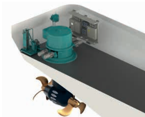
LM unit with integrated permanent magnet motor.
