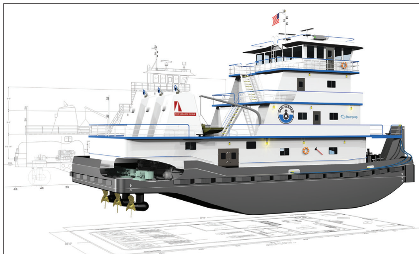
Stern view with cutaway showing Z-drive units.
