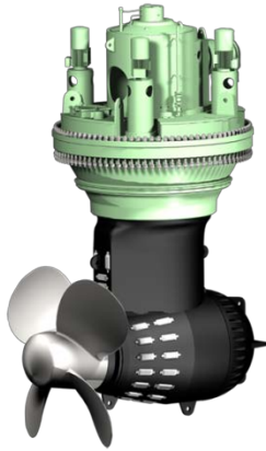
ii 3D model of the Steerprop SP O 4,5 ARC propulsor installed on the Varandey
